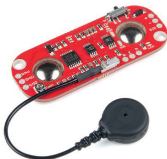
1-nji surat. MyoWare Muscle Sensor (AT-04-001) kysymly elektromiografiýa enjamy
